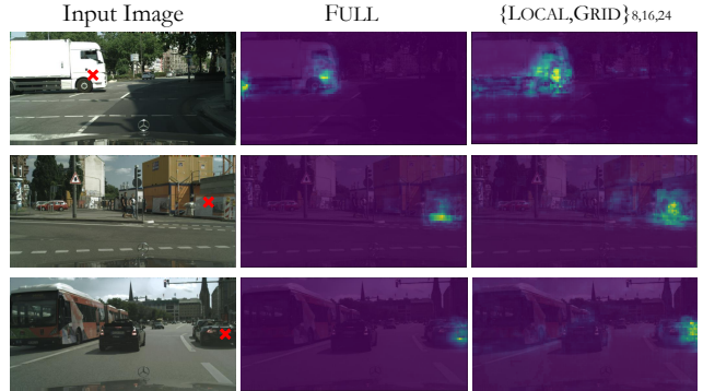
Figure 6: Comparing the receptive fields of the two models: FULL and the \{\text{LOCAL}, \text{GRID}\}_{8,16,24} with respect to the red \times in the input image. Larger values are visualized in higher brightnesses.
